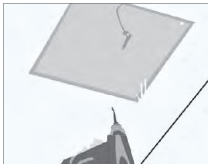
5. Fix securely using Drywall Screws and re-fit the door to check operation and then remove to allow for finishing Draw
